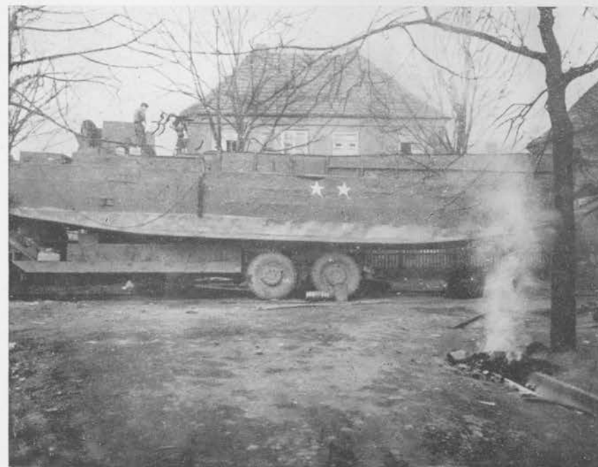
LCM LOADED ON M25 TANK TRANSPORTER
