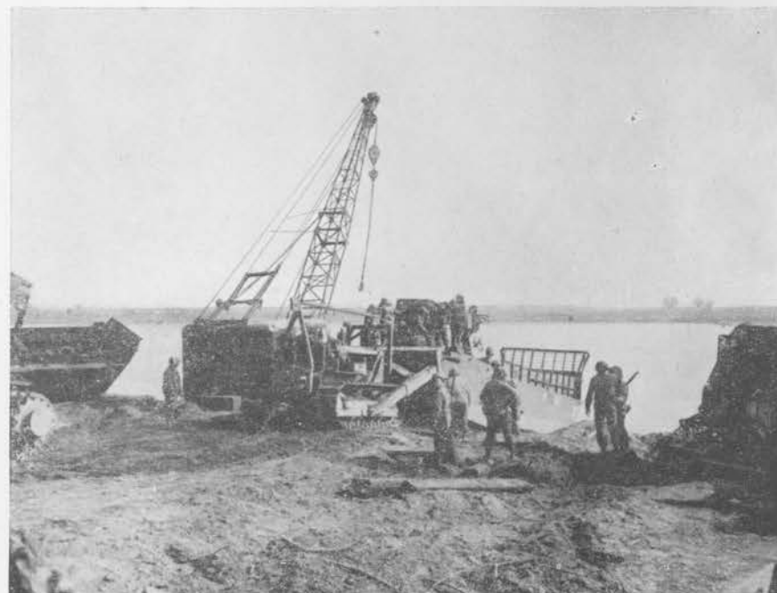
DOZER PUSHING LCM INTO WATER AFTER REMOVAL OF TANK TRANSPORTER
