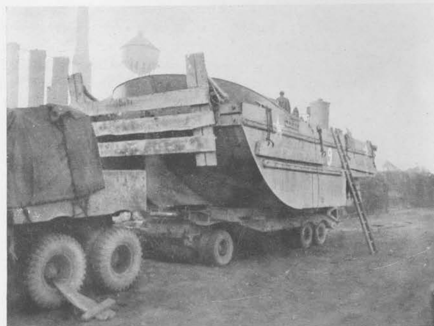
SEAMULE (COMPLETELY ASSEMBLED) LOADED ON M19 TANK TRANSPORTER
