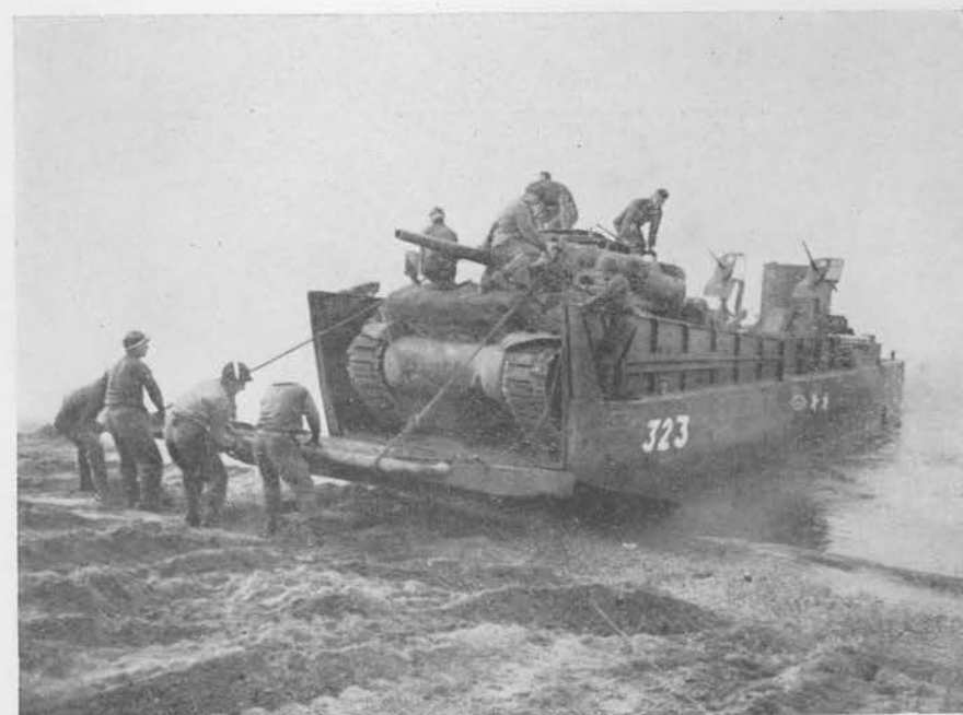
CLOSING DAMAGED END RAMP ON LCM BY MEANS OF ROPES ATTACHED TO M4 TANK
